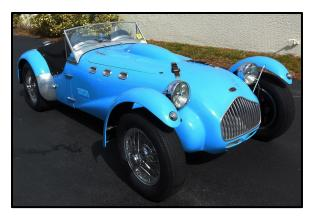
2123 was restored with a 390 Cad engine, Muncie transmission, Harden heavy duty rear hubs, and Halibrand quick-change rear end (for Bonneville). The J2 is located in Naples, Florida and is being offered for \$275,000 OBO. Interested parties should email allardregister@outlook.com. Please visit our web site for several photos and an extended history.
